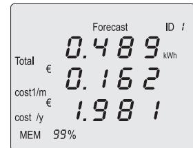
By pressing the „MODE“ key for at least 3 seconds, all displays of „Consumption“, „History“, „ON time“ and „Forecast“ are reset to nill, and the „MEM“ memory deleted.
