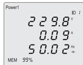
The maximum and minimum values are saved by the measuring device automatically. Via the „max“ (4) or „min“ (3) keys, the values are displayed for approx. 10 seconds. Pressing the key again switches back to the normal display prematurely.
