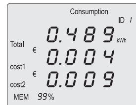
In order to read the preset tariff values for tariffs 1 and 2, press the „max“ key once. The display switches back after approx. 5 seconds.
