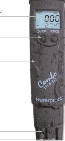
Replaceable pH electrode cartridge
