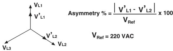
The voltage asymmetry causes the rise in motor temperature and a reduction of the rated motor power.
