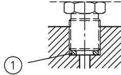
1 Cu sealing ring DIN 7603
