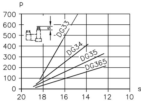
*p* pressure setting (bar); *s* adjustment dimension (mm)
