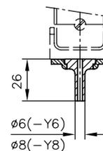
DG 3.. can be rotated in any direction around the pipe axis after loosening the clamping plate (by loosening M4).
