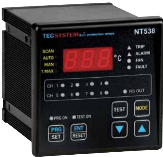
*Electronic microprocessor based unit for the temperature monitoring of electric motors and MV dry type/cast resin transformers. **The unit, due to the 8 input channels and the various programming options, grants a great flexibility of use in many applications.***
