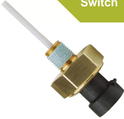
The **Model S85** is an active device which is designed to give an alarm signal if liquid falls below / rises above a preset level. It will only signal an alarm after a few seconds of low / high level to eliminate false alarms due to turbulence.
