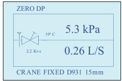
Unlike any other commissioning unit, the most commonly used functions – Flow and Pressure – are shown as the default screen from the Display menu. This means that for most general commissioning purposes the most valuable data is shown at the touch of a button – in large text.
