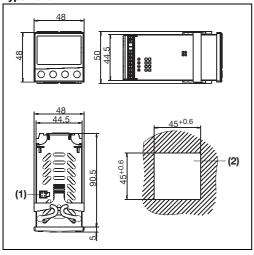
(1) PC interface adapter (setup connector)
