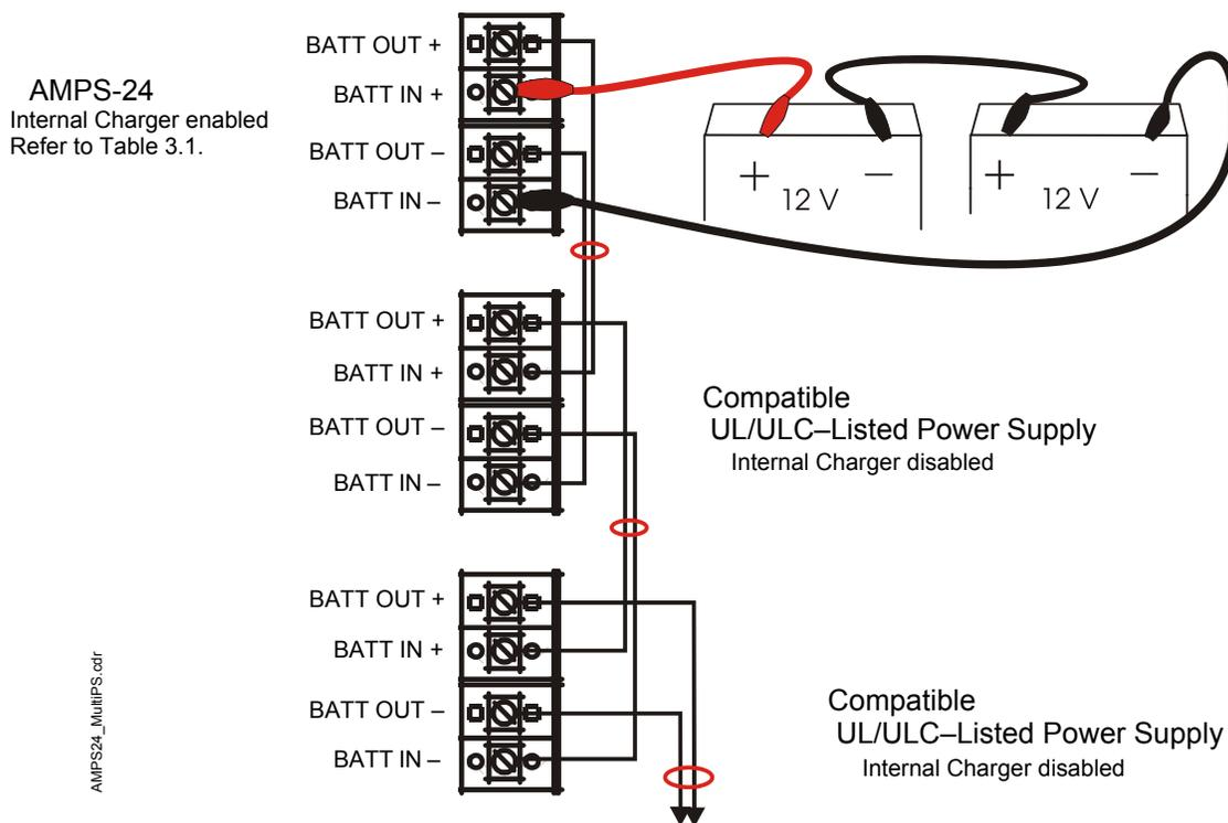
Figure 2.19 Connecting Multiple Power Supplies
