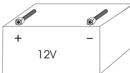
**Figure 2.14 Terminal Bolt Installation**
