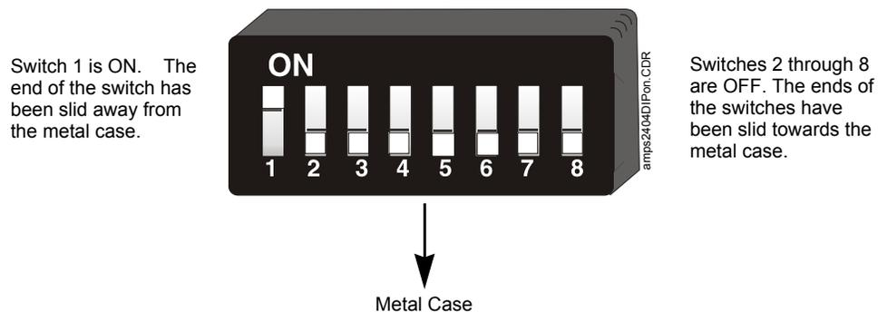
Figure 3.1 Setting a DIP Switch
