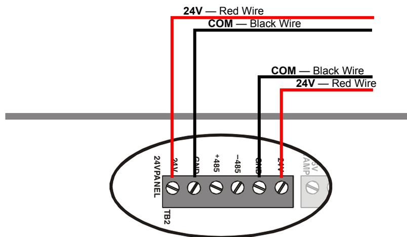
Figure 2.9 Connecting to the Panel Output TB2
