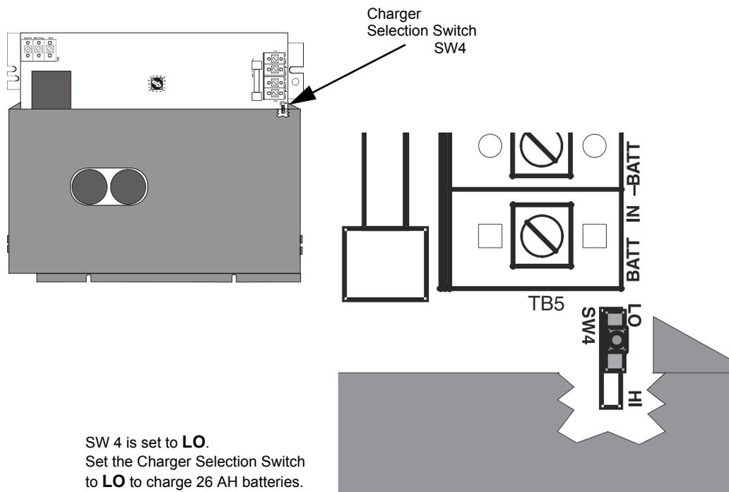
Figure 2.15 The Charger Selection Switch (SW4)
