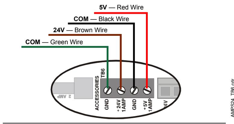
Figure 2.11 Connecting to the Accessories Output TB6
