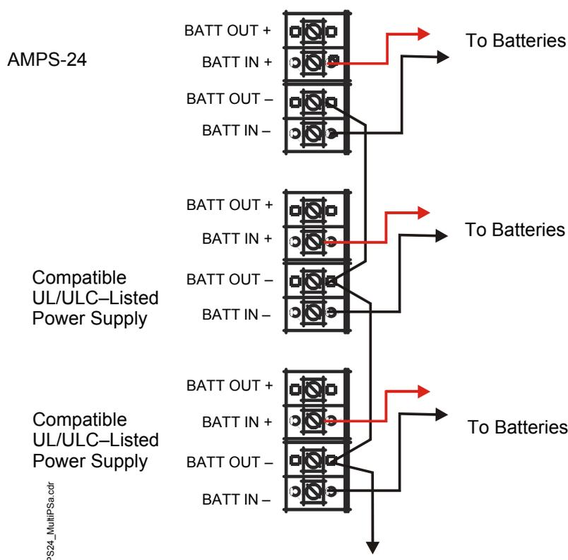
**Figure 2.18 Connecting Multiple Power Supplies with Common Bond Wire**
