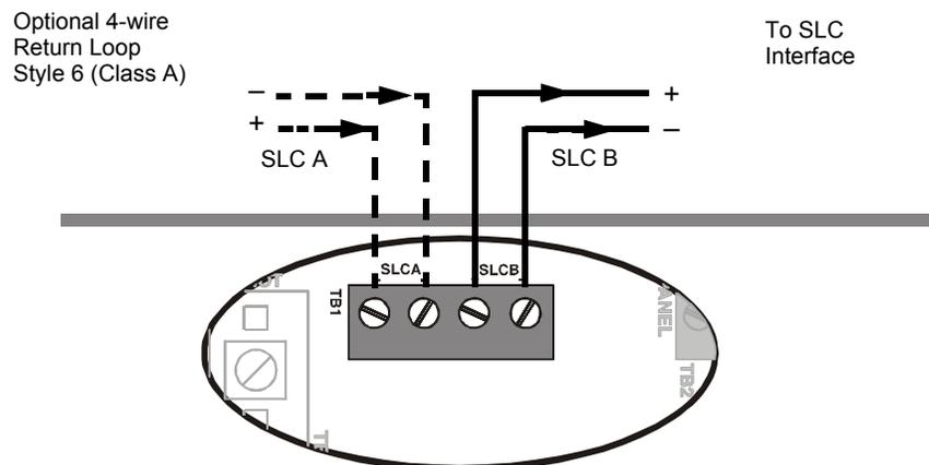
Figure 2.10 Connecting to the SLC Interface TB1
