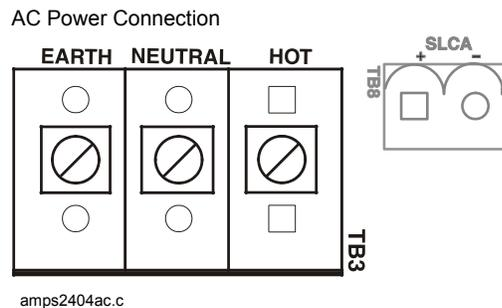
**Figure 2.12 AC Power Connection**
