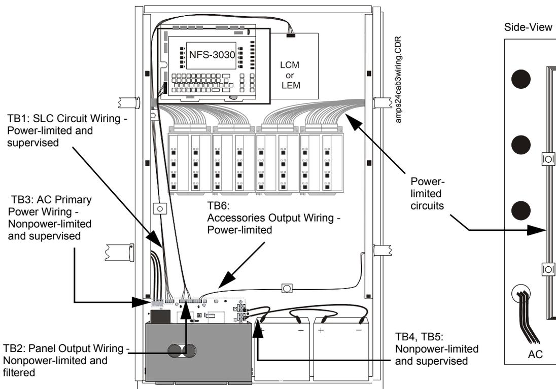
**Figure 2.6 CAB-4 Series Cabinet: Power-limited Wiring Example**
