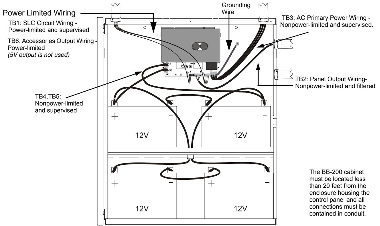
**Figure 2.8 BB-200 Cabinet: Power-limited Wiring Example with Four Battery Wiring**
