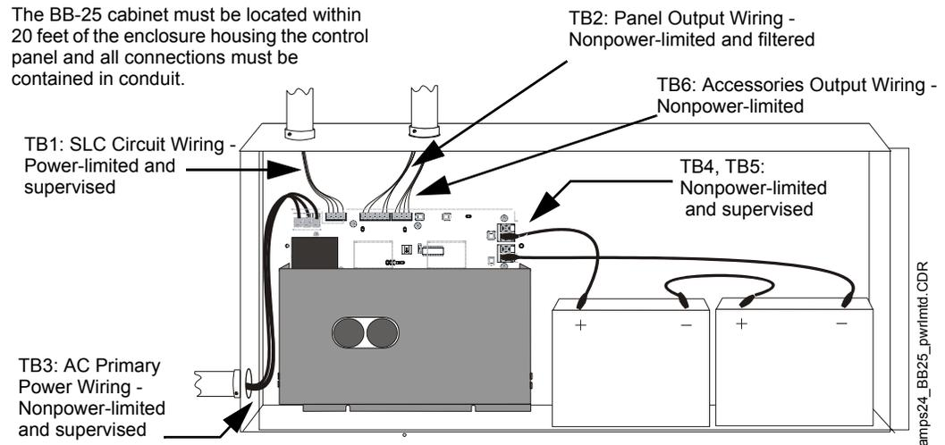
**Figure 2.5 BB-25 Cabinet: Power-limited Wiring Example, with Two Battery Wiring**
