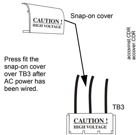
**Figure 2.13 Installing the TB3 Snap-on Cover**
