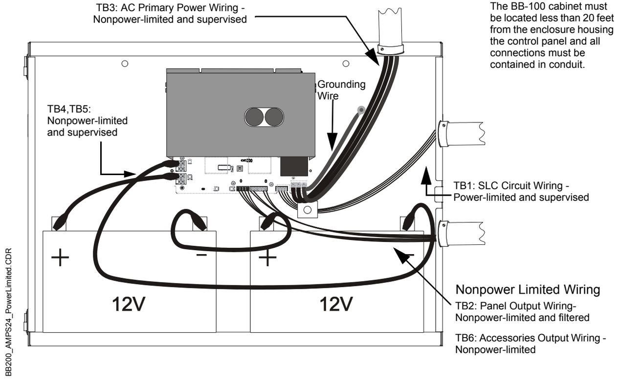
**Figure 2.7 BB-100 Cabinet: Power-limited Wiring Example with Two Battery Wiring**
