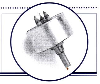
High quality container sealed, wirewound panel control of robust and reliable construction, with spindle and panel seals. Aluminium case and bushing; Anodized aluminium alloy spindle and fixing nut; locking washer; nickel plated brass lid; silver plated brass tags insulated from lid by ceramic standoffs.
