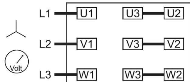
Double star connection, multi-voltage motor with 12 terminals (low voltage):
