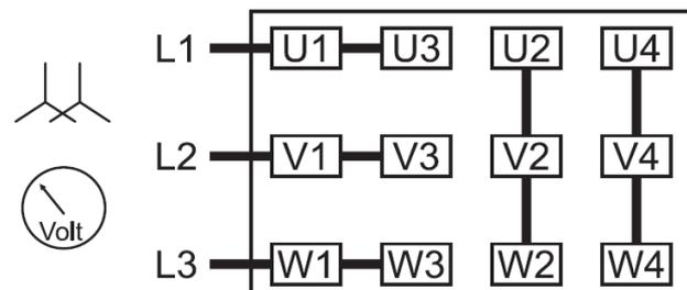
Delta connection, multi-voltage motor with 12 terminals (middle voltage):
