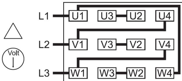
Star connection, multi-voltage motor with 12 terminals (high voltage):
