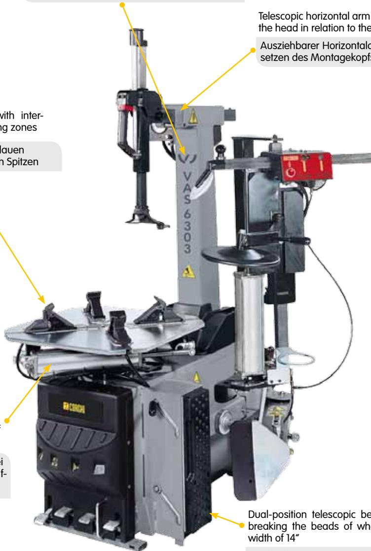
Dual-position telescopic bead breaker support for breaking the beads of wheels up to a maximum width of 14"
