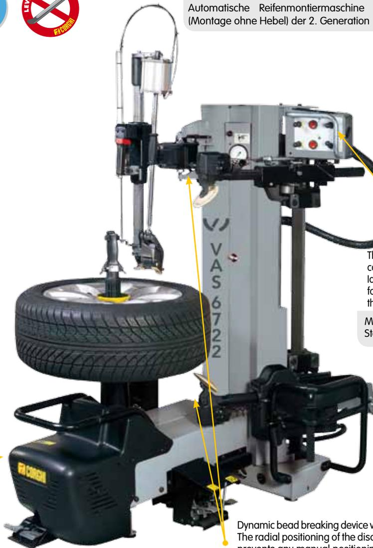
The multifunctional control console contains all the operating controls. Ideal for dynamic bead breaking and for rim and tyre match mounting, thanks to the two dual control discs.
