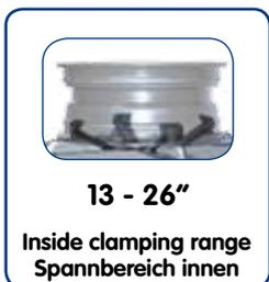
New turntable system with two pneumatic cylinders capable of clamping any type of rim securely
