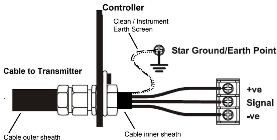
Diagram 9: Controller Grounding
