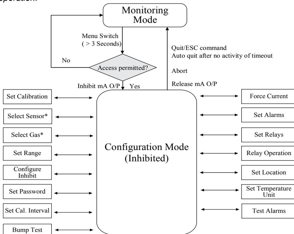
\* Note : "Select Sensor" and "Select Gas" menus are only available for flammable/IR sensors.
