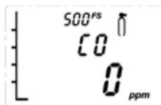
6. When the zero gas reading is stable use '✓' to confirm zero calibration.
