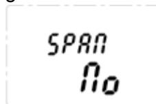
10. If span calibration is required use '✓' proceed to the next step. If span calibration is not required, use '▲▼' to select 'No' and '✓' to return to configuration mode.
