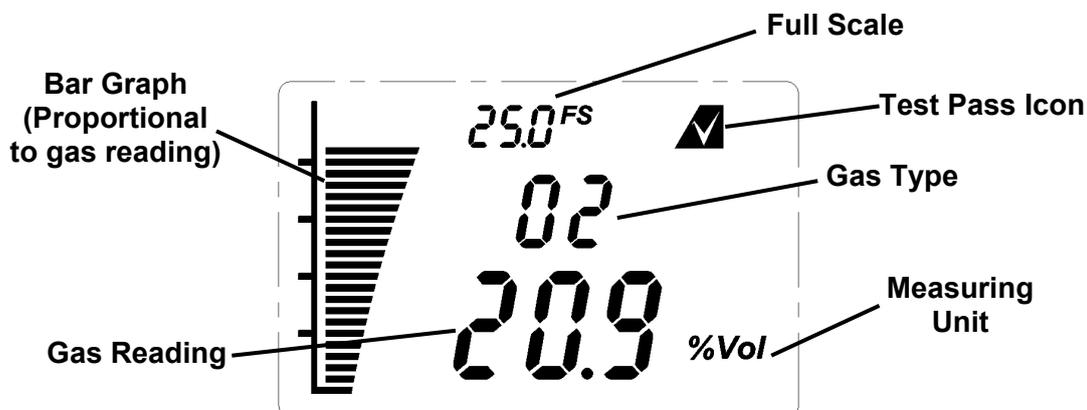
Diagram 11: Example of a O<sub>2</sub> Transmitter Display screen – Normal Operation
