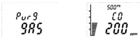
19. Promptly switch off the calibration span gas and remove the Sensepoint XCD Gassing Cap from the sensor to allow the gas to disperse.
