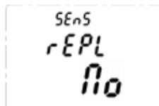
16. Use '▲▼' to select 'YES' if the sensor has been replaced or 'No' if it has not been replaced.
