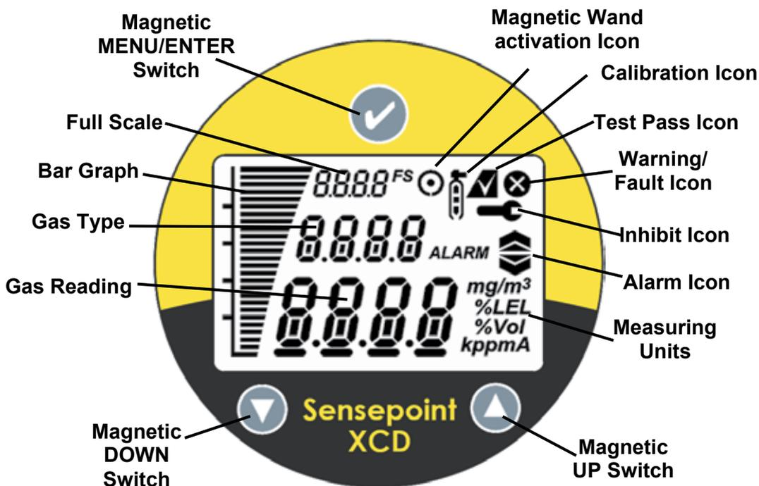
Diagram 2: Sensepoint XCD Display and Magnetic Switches
