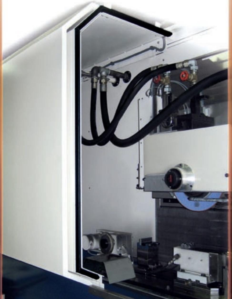
/// The potential hazards emanating from shear and pinch edges in machinery and plant construction facilities are many and various, and involve all sectors, from the automotive industry, to the steel and woodworking industries, all the way through to the plastics industry. Typically dangerous areas are lifting tables and work platforms, automatically operated doors at turning, milling and welding stations, plus machining centres, and protective hoods on presses and punches.
