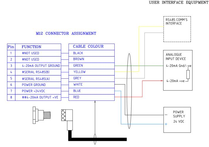
1MTR CABLE WITH M12 CONNECTOR SUPPLIED AS STANDARD. #USER TO SUITABLY INSULATE ANY UNUSED WIRES. RS485 IS AVAILABLE IF REQUIRED BY USER. ## THE 4-20mA IS A SOURCE OUTPUT.
