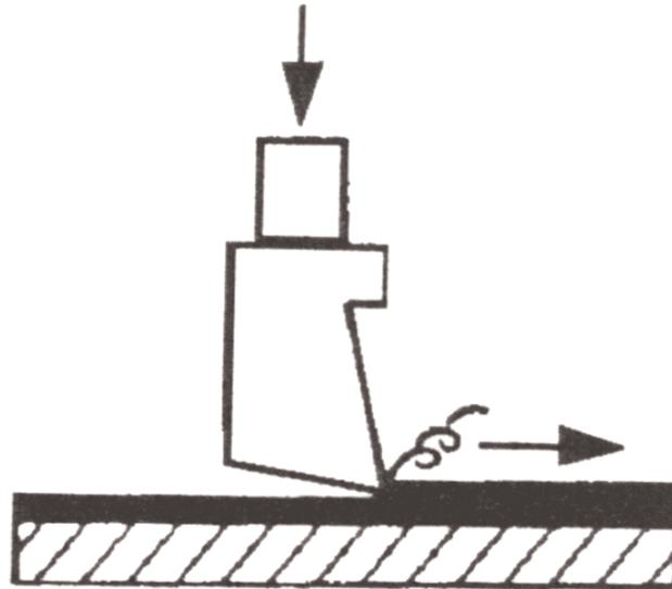
*Scratch Tool: Test Tip acc. to Clemen*
