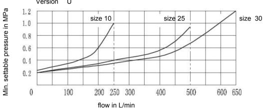
The characteristic curves are valid for outlet pressure B = 0 over the entire flow range!
