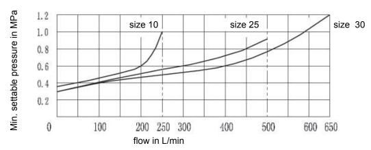
Minimum settable pressure and bypass pressure in relation to the flow Version  $\,\,^{''}\text{U}^{\,''}$
