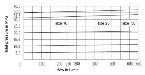
Minimum settable pressure and bypass pressure in relation to the flow Standard version
