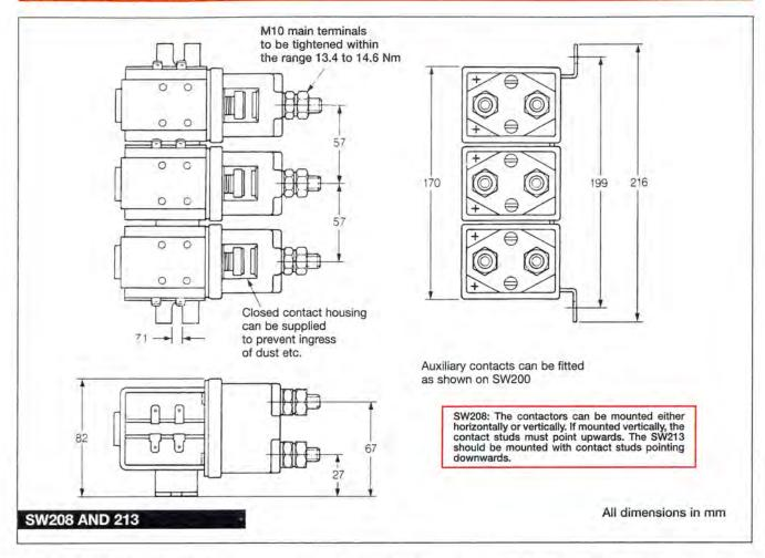
Pull-in voltages are approximately 60% and 66% of the rated voltage for intermittent and continuously rated types respectively.
