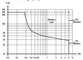
**Mechanical / Electrical life:**  $5 * 10^6 / 3 * 10^4$  operation, typical. **Operate / Release time:** 8 / 4 ms typical. **Bounce time NO / NC contact:** 3 / 8 ms, typical.
