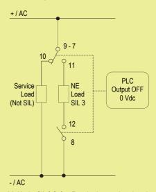
Contacts 7-11 and 8-12: the SIL 3 Safety Function is met when the relays are de-energized, contacts are open, NE load is de-energized.
