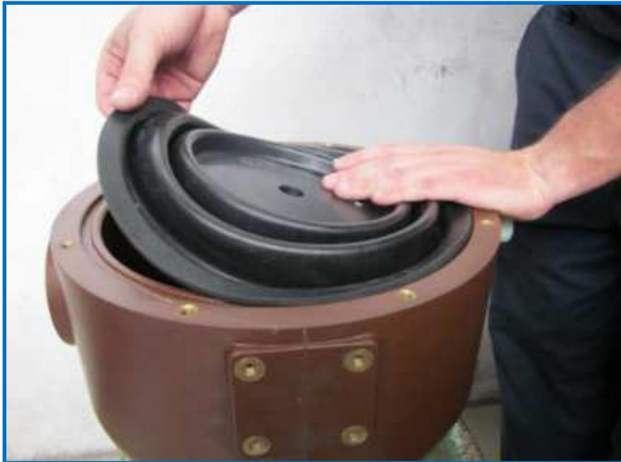
7. Fix the M8 screws to 20 Nm. that hold the aluminium flange which at the same time is holding by pressure the new aluminium flange and the new rubber bellows in place.
