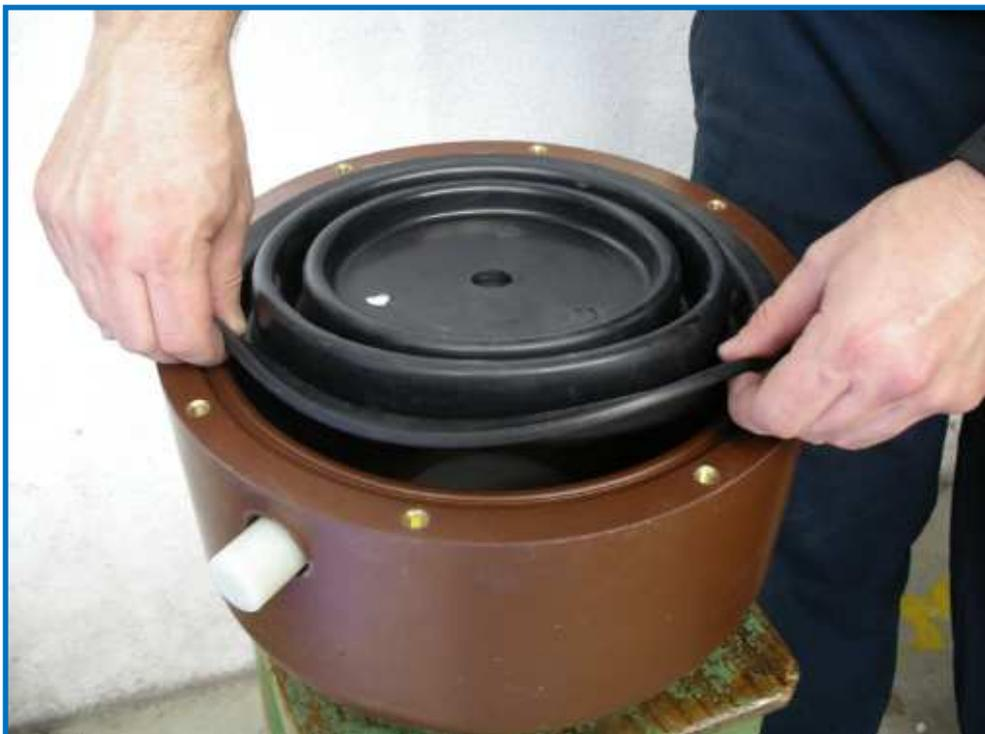
6. Place the new rubber bellows (code 452025638) as seen in the photo, applying pressure with one hand in the central part, forcing it to be in contact with the oil, while at the same time allowing the air to flow out the open part.
