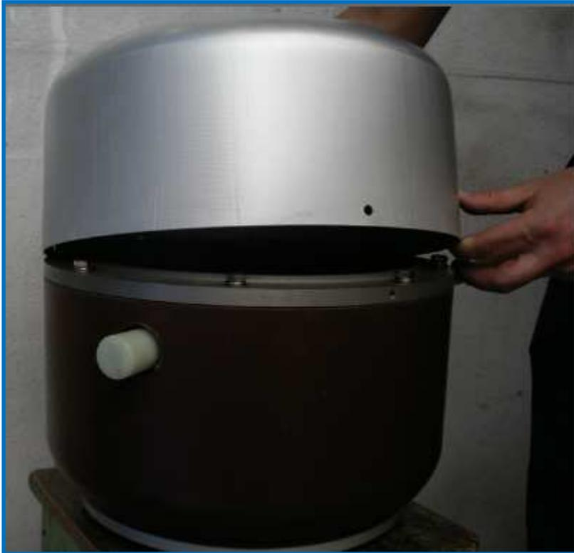
3. Once the cover is removed, loosen the M8 screws that hold the aluminium flange (code 432104347) which at the same time is holding by pressure the rubber bellows in place.
