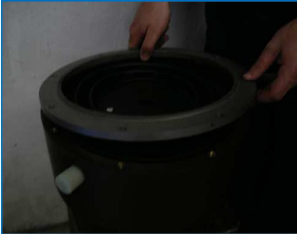
5. Remove the rubber bellows (code 452025539) by hand, with a quick movement, to avoid any part of it sinking into the oil.
