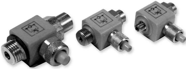
These valves are used to regulate exhaust airflow. For example: to control the piston on double-acting cylinders. An adjustment screw allows variable flow in one direction (arrow) and permits air to flow freely in the opposite direction. These space saving valves mount directly into the cylinder port. The body can be rotated 360° for optimum alignment.
