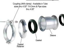
Self-restrained gaskets are used in vibration applications to prevent coupling "walking" on the pipe, or in applications where there is thermal expansion or poorly anchored piping systems.
