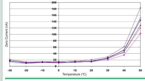
Figure 3 shows the variation in zero output of the working electrode caused by changes in temperature, expressed as nA.
