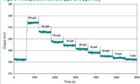
Figure 4 Response from 200 ppb to 0 ppb NO<sub>2</sub>
