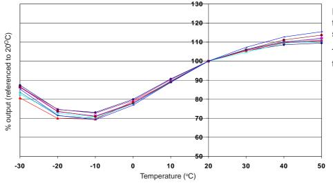
Figure 2 shows the temperature dependence of sensitivity at  $2ppm NO_2$ .
