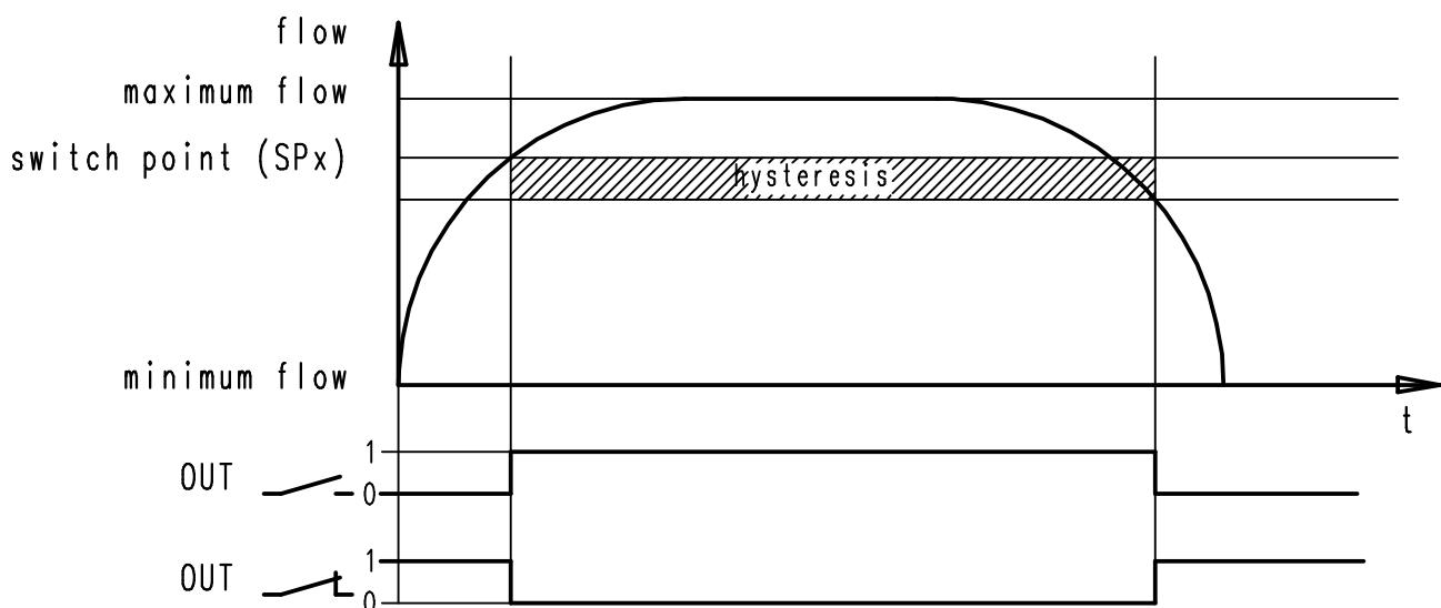
When the flow rises, the outputs switch when the corresponding switch point (SPx) has been reached. When the flow falls again, the output switches back when the value 'SPx - hysteresis' has been reached.
