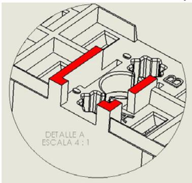
The sockets have star-shaped sockets as shown in the following figure which allow a large number of combinations.
