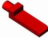
These Security pins are placed in the sockets and in the relays to allow the client/user to code the relays and sockets to avoid errors when replacing relays already installed so that only a correct relay model can be connected (e.g., RF-4 OP00001 for 125 V DC).
