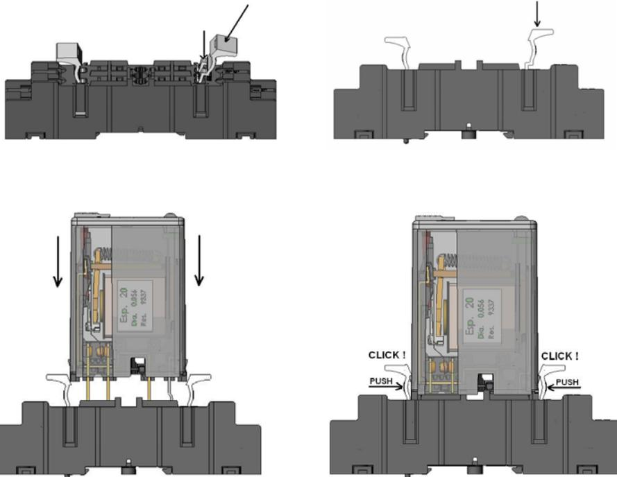
To remove the relay, release the retaining clip by pressing lightly on it as shown in the following figure.
