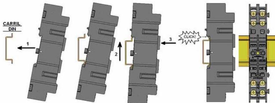
To remove a front socket from a DIN rail:
