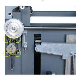
7. Disconnect the motor lead. This connector is in the inside of the machine. Pull the entire assembly out.
