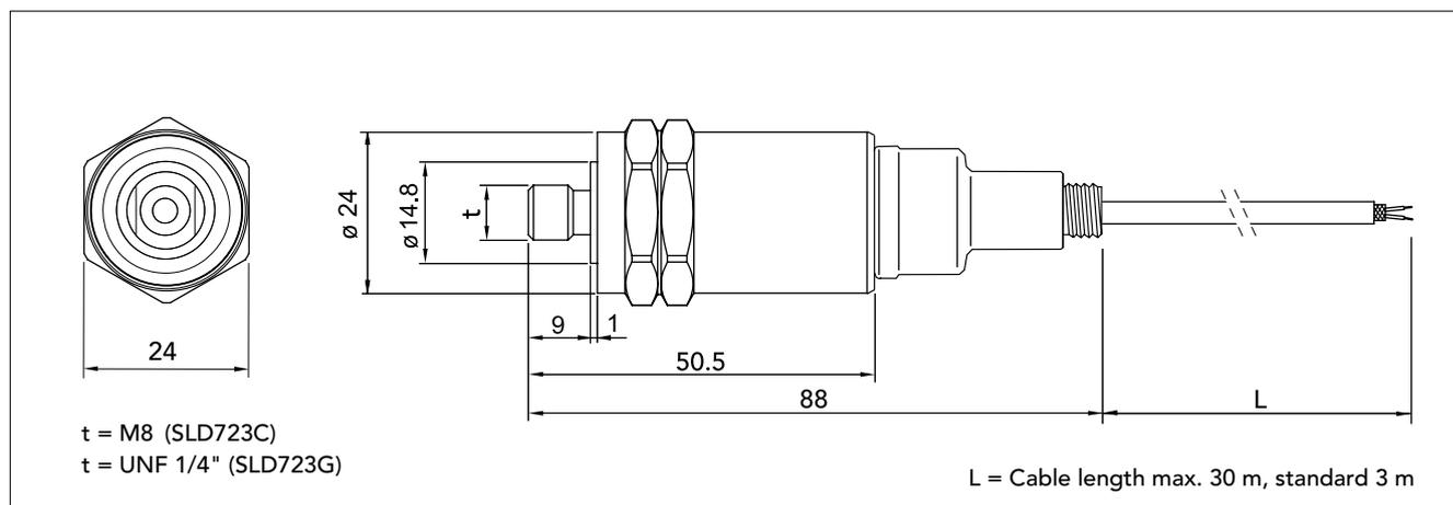
The 4-20 mA vibration transmitters are piezo-electric accelerometers of compression type and provide a 4-20 mA output signal proportional to the true RMS value of vibration velocity. The transmitters can be connected to common process control systems (PLC, DCS). The electrical signal is isolated from the transmitter housing. The transmitter operates by using power from a standard 4-20 mA loop.
