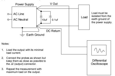
Figure 3-2 Ripple Noise Measurement Setup
