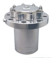
MKII 80mm Internal Gas Relief Valve & Bursting Disc Holder- Suitable for a pressure range of between 100 - 505 PSI (6.90 - 34.82 bar). Contact parts manufactured in 304/316 stainless steel. Fitted with PTFE seals as standard.
