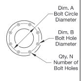
FIGURE 3 GATE VALVE FLANGE NOMINAL DIMENSIONS
