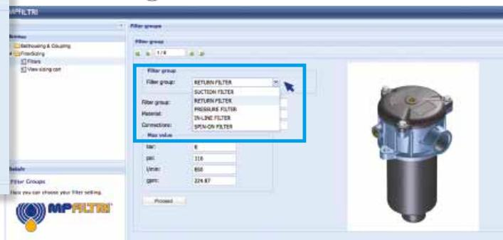
**Step 3** Choose filter type (MPF, MPT, etc.) in function of the max working pressure and the max flow rate
