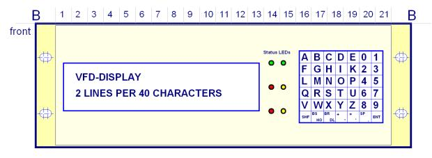
(here with option "BG7008/6LED" - front panel for system 7001RC including 6x status LED)
