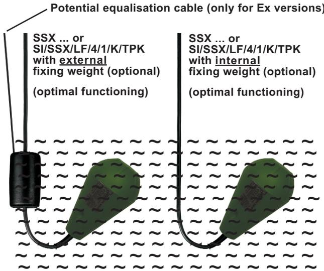
These floating switches are designed for mounting from the side or from the top.
