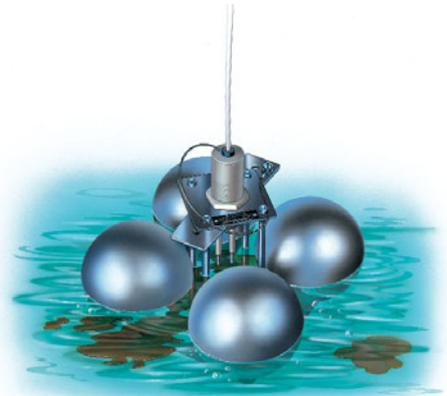
If, for example, oil flows onto a still water surface following a leak, exact setting of the rod electrode will ensure that an oil layer of only approx. 3 to 10 mm thickness is sufficient to interrupt the control current flowing via the rod electrode and activate an alarm.
