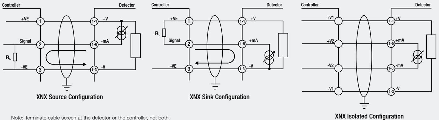
Note: Terminate cable screen at the detector or the controller, not both.
