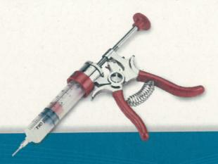
The AD93 volumetrically dispenses epoxies, silicones, glues and pastes. Available in two capacities, 35cc and 80cc syringe, with hot stamped sidewall indicators for dosage levels in cc and ounces. Shot sizes can be selected in increments of 1cc to 5cc. Material delivery is via luer lock tips.
