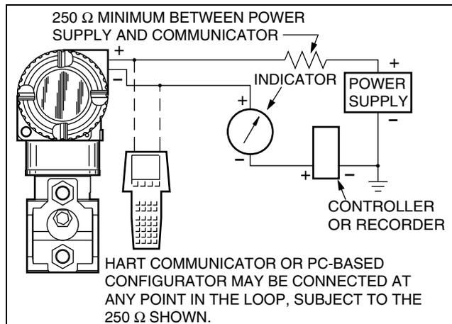
Figure 20. 4 to 20 mA Output Block Diagram
