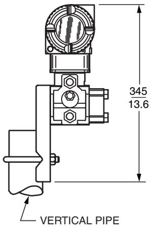
TRANSMITTER WITH LOW PROFILE STRUCTURE LP2
