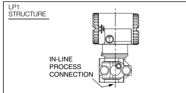
Figure 7. Low Profile Structure - LP1 Shown
