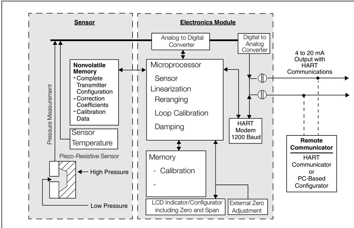
Figure 17. Transmitter Functional Block Diagram
