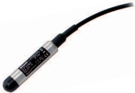
**Hydrostatic level meter HLM-25S** is compact measuring device containing silicon strain gauge sensor and evaluation electronics in stainless steel probe. From the probe housing comes out 2-wire cable with capillary (for atmospheric pressure compensation). The front side of the sensor is equipped with plastic removable cap (to avoid membrane damage). The level meter has no customer-accessible adjusting elements.
