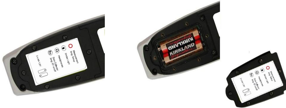
For installing new batteries, please remove all empty batteries first, before installing new or fully charged batteries. Always assure the correct battery orientation shown on the battery cover label. Pay attention to the proper fit of the rubber gasket, before closing.
