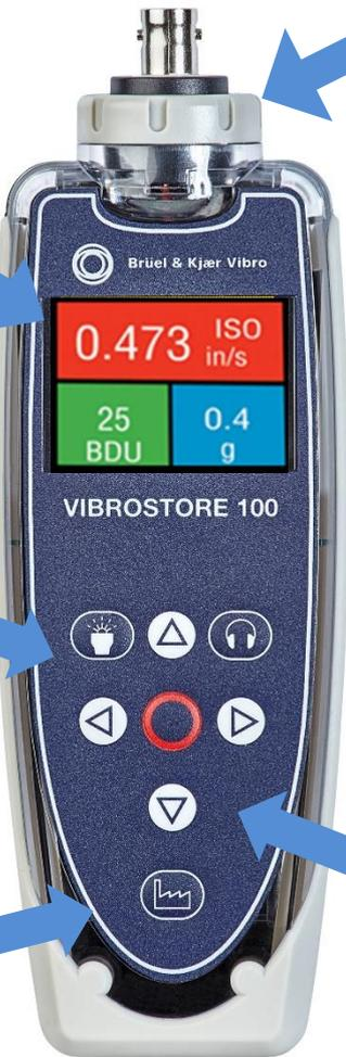
Press and hold the **centre** button
