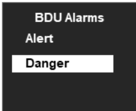
The default BDU thresholds are 50 for **ALERT** and 100 for **DANGER**. These levels are typical for medium sized machine bearings operating at run speeds in the region of 1000 to 3000 RPM. Larger bearings or higher run speeds may need increased BDU threshold values to identify worn or bad bearings.
