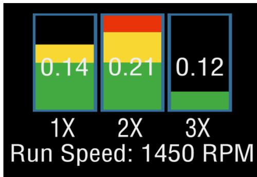
N.B. in order to perform a vibration analysis it is important that the running speed of the machine is entered correctly. This can be done with the “Setup Wizard” as described in Section 3.5.1 of this user guide, or by using the strobe attachment (see Section 6.1)
