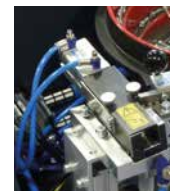
Escapement sensors Control/Secure escapement mechanism
