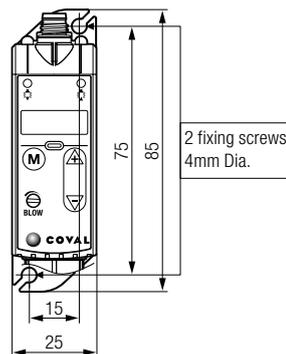
For fixing from front, please order the necessary kit in addition to the ejector module:
