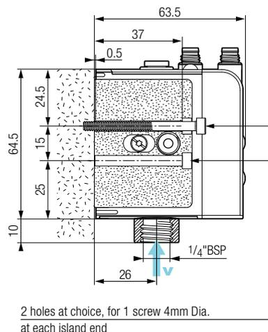
2 holes at choice, for 1 screw 4mm Dia. at each island end
