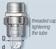
These threaded cap fittings are available into the COVAL catalogue : elbows, Ys, manifolds and straight threaded connectors (illustration), for  $d \times D$  tubes (4 x 6 mm, 6 x 8 mm and 8 x 10 mm).
