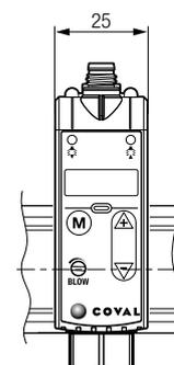
The module may be clipped over a DIN rail.
