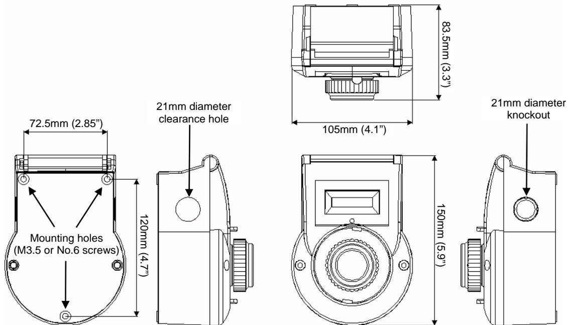
Diagram 2: Detector dimensions and mounting hole locations
