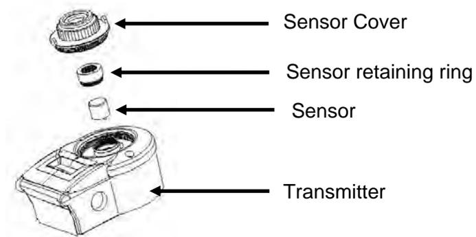
Diagram 7: Replacing plug in sensor
