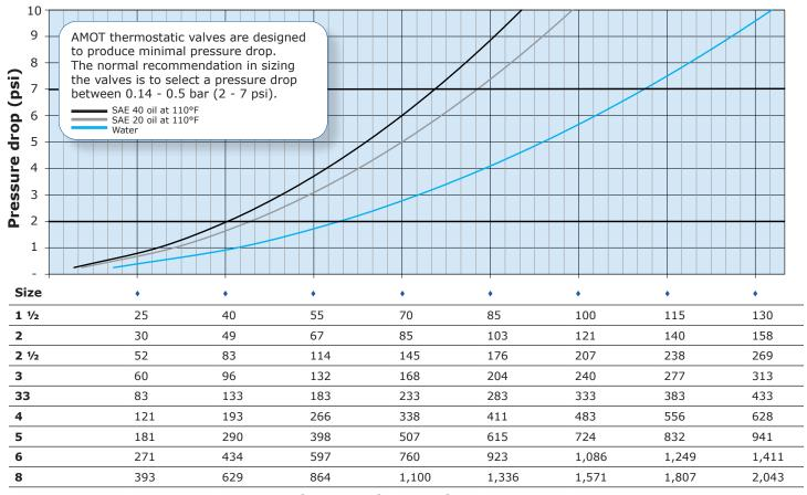
Flow rate (US gpm) - Water
