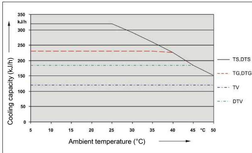
Remark: The limit curves for the heat exchangers exchanger apply to a dew point of 65 °C.
