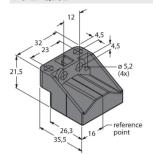
Floating positioning element for Li-Q25L linear position sensors; operational at an offset of 90; nominal distance to sensor 1.5 mm; pairing with linear position sensor at a distance of up to 5 mm; misalignment tolerance of up to 4 mm
