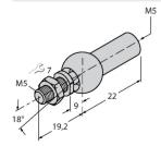
Axial joint for guided positioning element, stainless steel
