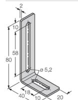
Mounting bracket and sliding block for linear position sensors LI-Q25L; material: Stainless steel; 2 pcs. per bag
