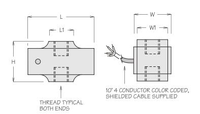
Rated Output (R.O.): 2 mV/V nominal Nonlinearity: 0.1% of R.O. Hysteresis: 0.1% of R.O. Nonrepeatability: 0.05% of R.O. Creep in 20 Min.: 0.05% of R.O. Zero Balance: 1.0% of R.O. Compensated Temp. Range: 60° to 160°F Safe Temp. Range: -65° to 200°F Temp. Effect on Output: 0.005% of Load/°F Temp. Effect on Zero: 0.005% of R.O./°F Terminal Resistance: 350 ohms nominal Excitation Voltage: 10 VDC
