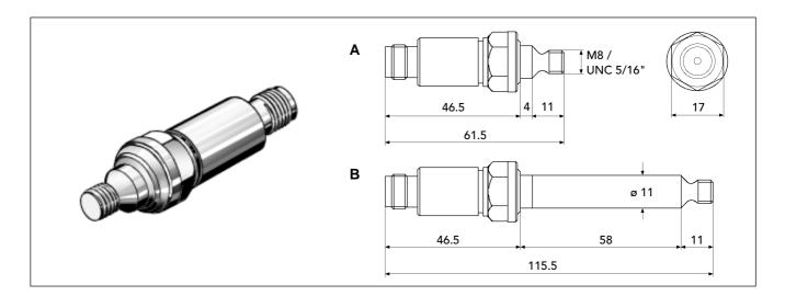
Standard shock pulse transducers are used in all permanent SPM installations for bearing monitoring. They are installed in countersunk mounting holes on the bearing housings.
