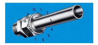
3. Hold the fitting body steady with a backup wrench and tighten the nut 11/4 turns. Watch the scribe mark, make one complete revolution and continue to the 9 o'clock position. When the nut is tightened to the 9 o'clock, you can easily see the fitting has been tightened properly.
