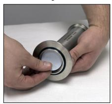
Photo 3: Membrane Filter Insertion
