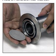
5. Fit the cell bottom onto the cell body, aligning the circular groove with the circular ridge on the bottom of the cell body (Photo 5).
