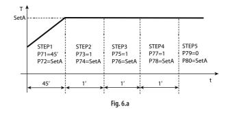
At the end of Step5, the operating cycle ends automatically and control resumes based on Set1.
