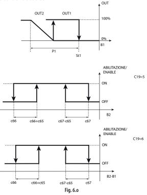
Direct" control with enable logic:
