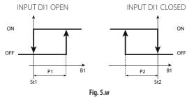
Modes 7 and 8. The outputs with "dependence"=17 will have the effect shown in the figure when ID1 switches.
