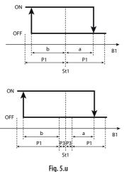
The PWM (or analogue) outputs will follow the operation indicated in the figure. In practice, in the dead zone the output maintains the level of activation unchanged.
