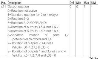
Rotation 2+2 on 4 outputs (c11=2) has been designed to manage capacitycontrolled compressors. Outputs 1 and 3 activate the compressors, outputs 2 and 4 the capacity control valves. Rotation occurs between outputs 1 and 3, while the valves are energised (relays ON) to allow the operation of the compressors at maximum capacity. Valve 2 is linked to output 1 and valve 4 to output 3.
