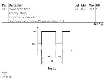
igvarboxAs the action of PWM operation is modulating, PID control can be fully exploited, so that the value coincided with the set point or falls inside the dead zone
