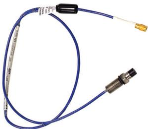
The MX8030 and MX2030 probe series consist of 5mm and 8mm tip diameter probes. The MX8030 comes standard with triaxial cable and VibeLock™5 connector. The MX2030 comes standard with a coaxial cable and rounded knurled connectors. Both probes offer a full 80 mil (2mm) range, and are designed to offer full API 670 compliance when used with a matching MX8031 or MX2031 extension cable and a MX2033 driver or a MX2034 transmitter.
