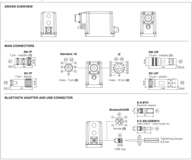
(1) Use of metallic connectors is strongly recommended in order to fulfill EMC requirements
